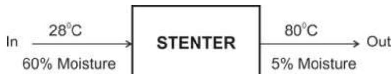
The heat input to the stenter is provided by a thermic fluid heater fired by fire wood as fuel. Gross Calorific Value (GCV) of Fire Wood is 3500 kcal/kg. The efficiency of the thermic fluid heater is 70% and distribution loss in the thermic fluid system is 20,000 kcal/hr. The average
